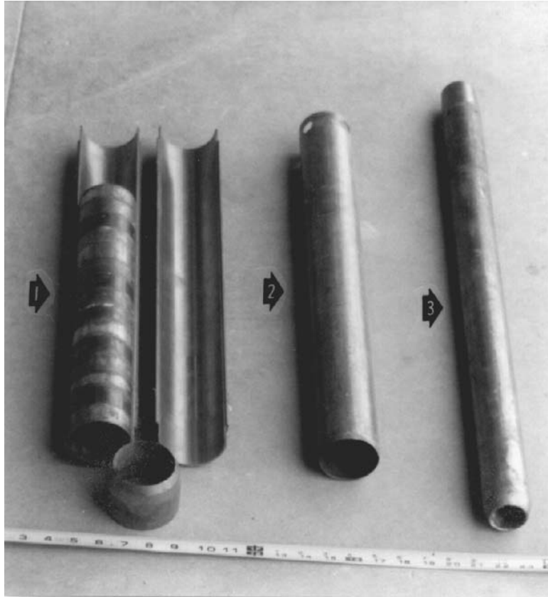
FIGURE 2.10 Soil samplers (no. 1 is the California sampler in an open condition, no. 2 is a Shelby tube, and no. 3 is the standard penetration test sampler).
