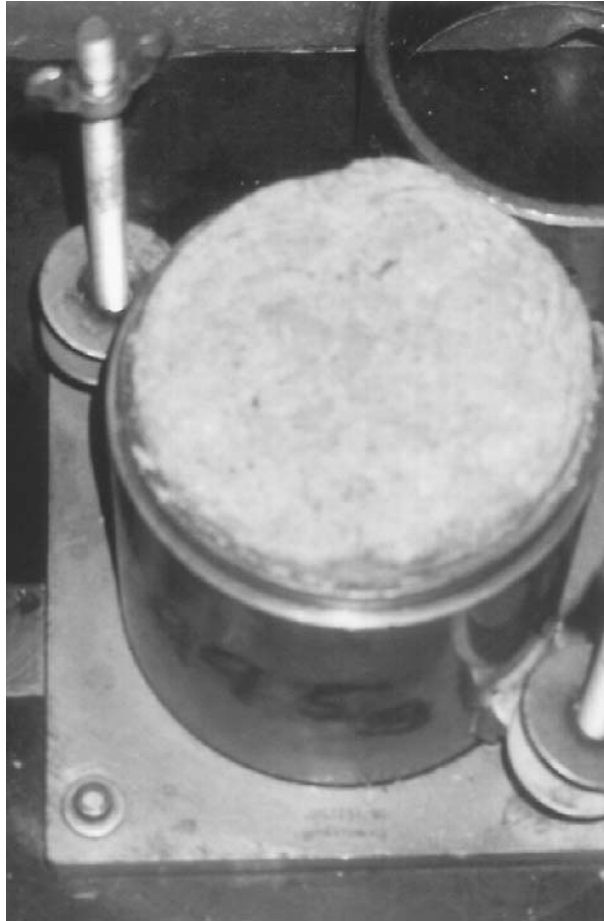
FIGURE 3.49 Completion of the compaction test with the top collar removed.
