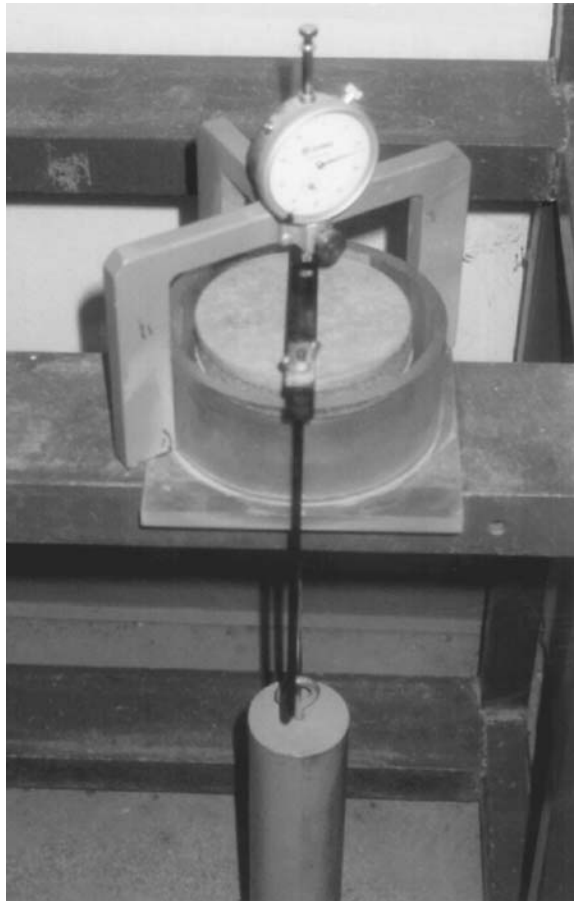
FIGURE 9.6 Example of a loading device for the expansion index test.
