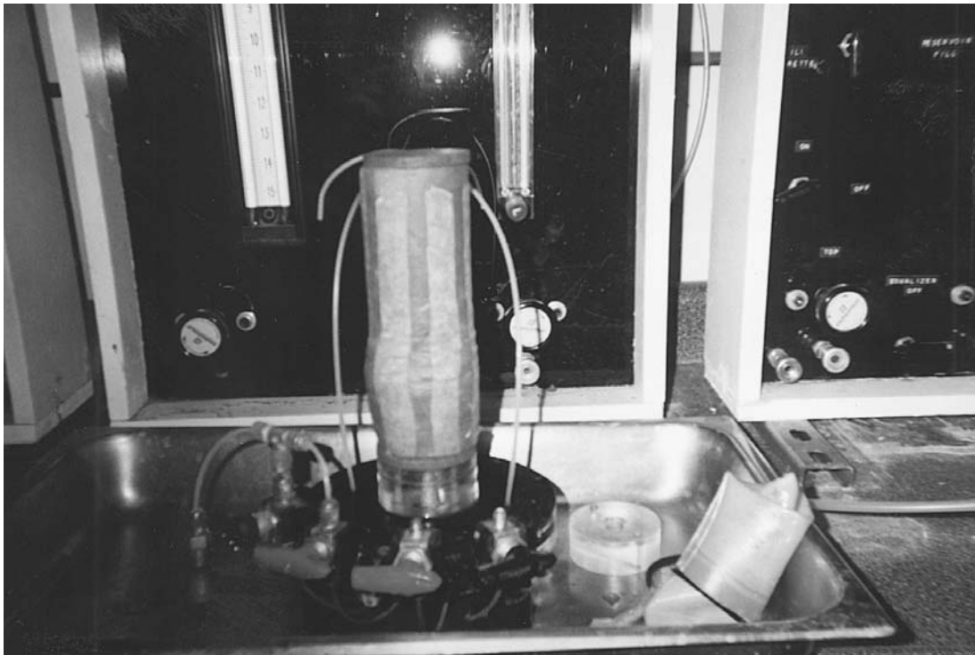
FIGURE 3.26 Bulge-type failure condition of the soil specimen.
