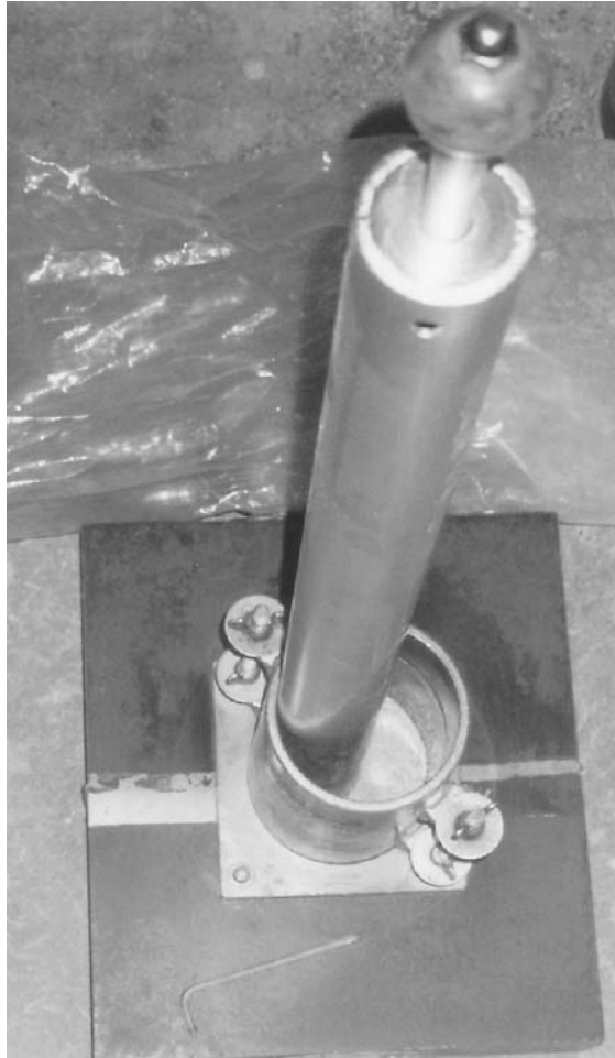
FIGURE 3.48 Soil in the process of being compacted into the compaction mold using the Modified Proctor rammer.
