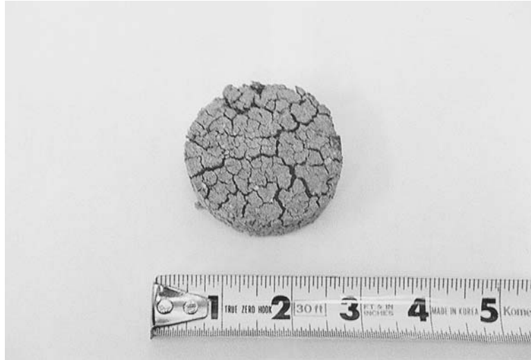
FIGURE 9.18 Specimen of desiccated Otay Mesa clay.
