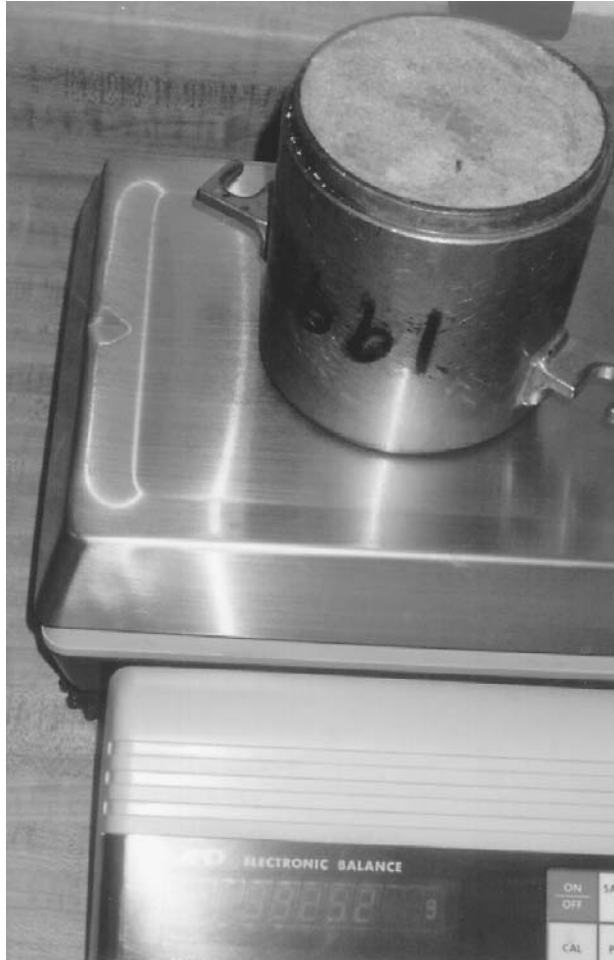
FIGURE 3.50 A balance is being used to determine the mass of the mold plus compacted soil.
