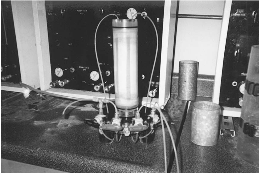
FIGURE 3.23 The soil specimen and specimen cap have been placed on the base plate pedestal, the soil specimen has been sealed with a rubber membrane, and the O-rings are in place.
