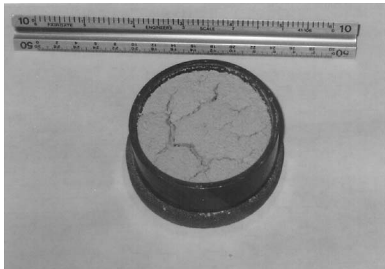
FIGURE 9.12 Soil specimen that has been air dried to a water content below the estimated shrinkage limit and is ready for testing.
