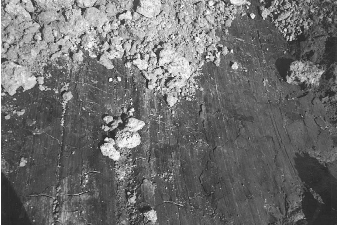
FIGURE 3.44 Photograph of the slide plane, which was exposed during the stabilization of the Niguel Summit landslide. Note that the direction of movement of the landslide can be inferred by the direction of striations in the slide plane.
