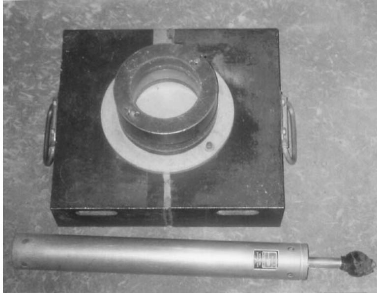
FIGURE 9.4 Mold attached to a rigid anchor block.
